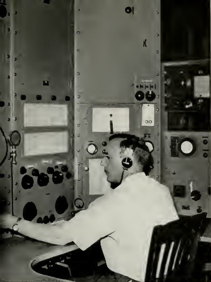
Technician F. B. Kennell at the main operating position of RCA's frequency Measuring Laboratory tunes in a radio station which is to be checked for accuracy of transmissions.
