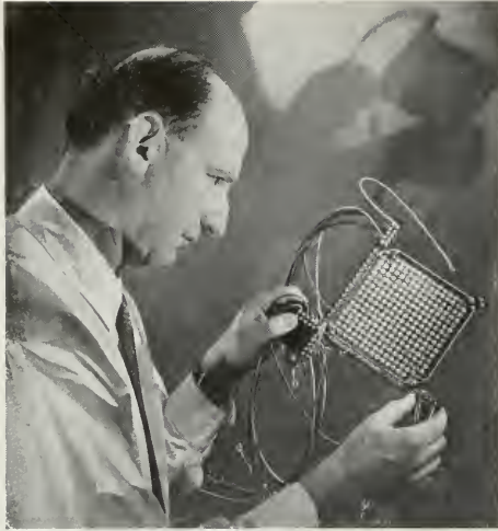
Dr. Jan A. Rajchman holds one of his Myriabit Magnetic Core Matrix Memory units which is capable of retaining 10,000 bits of information until needed.
